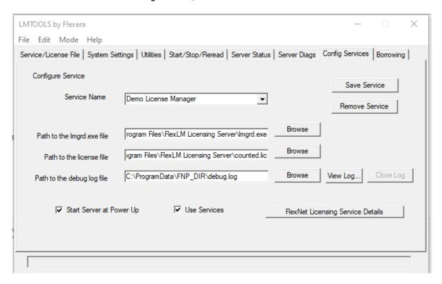
Figure 10-1: Completed Config Services Tab
